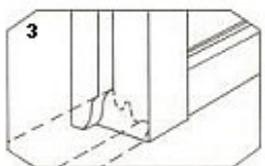
**3** Chisel out sufficient from the bottom of the frame on both sides to receive the inside face of the door sill, shaping the cut to the profile of the front of the door sill (fig 3).
