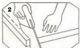
**2** Remove the door from its hinges and saw along a line parallel to the mark and 3mm above it to allow 3mm clearance between the door bottom and the outside upstand of the door sill. Smooth down the sawn surface with sandpaper. For ideal operation gloss paint or varnish the surface to ensure surface is smooth.
