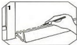
**1** If necessary cut the door sill to the correct length i.e. the exact width of the door frame opening. This will normally be a fraction wider than the door itself. Place the lower outside edge of the door sill against the inside face of the door when in its closed position, and mark along its length with as sharp pencil or marking tool.
